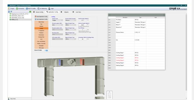
Looking for a fast way to check the configuration using Onyxx LX controllers? The I/O table updates live. In the Live view you can override any of the points to test the sequences ie: manipulate the zone temperature to a value above the cooling setpoint to verify the cooling sequence responds as desired. Same goes for any points.
